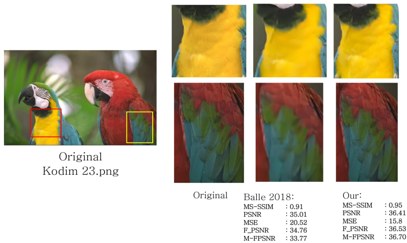
Fig. 5. Qualitative comparison results using the Kodak dataset between original data and using AB. Kodim 23.png Left: Original, Middle: Balle 2018, Right: ours.
